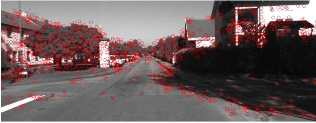
Figure 7: The keypoints detected in the first frame of KITTI seq05 sequence by SURF detector.
