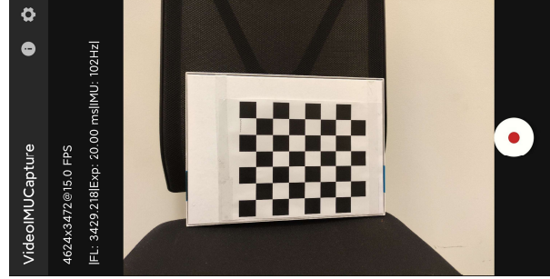
(b) The screenshot of the VideoIMUCapture app. The data is recorded with 4624x3472 pixels @15.0 FPS
